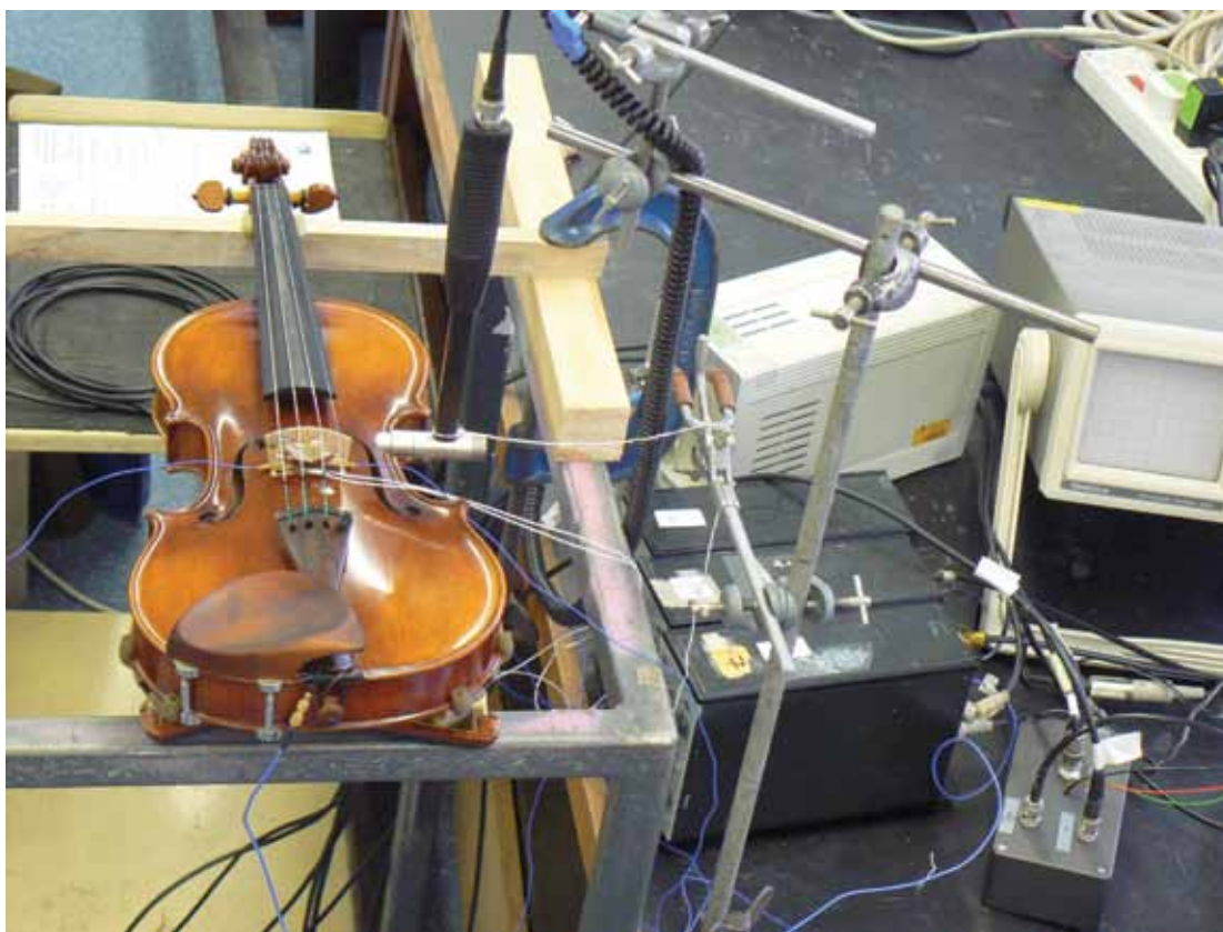
Figure 1. Photograph of the test rig showing the method of mounting the violin, the suspended hammer, the instrumented bridge with two white leads, and the instrumented tailpiece with a single blue lead. The two blue leads coming from the base of the bridge were not there during the experiment and relate to another project run at the same time, which involved measuring the accelerations at the bridge feet. The “sum and difference box” for the bridge transducers is seen at the bottom right corner.
